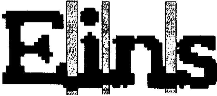
Fig. 9.4: The German word “Eins” with an indication of where it should be cut to separate the individual letters.
