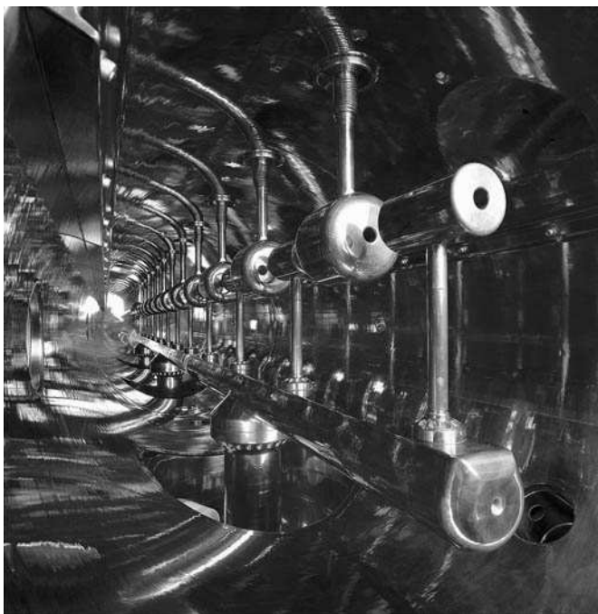
12. The particle accelerator used at the Institute for Heavy Ion Research (GSI) in Darmstadt, Germany, for fusing atomic nuclei to make new superheavy elements. The GSI team have used this equipment to make all the elements from 107 to 112
