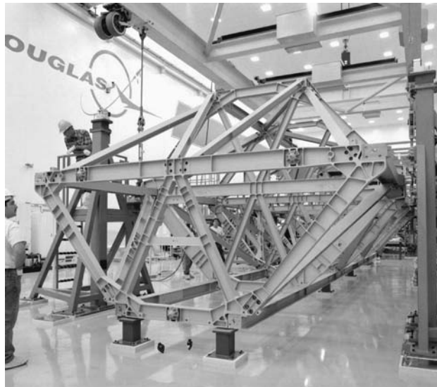
Fig. 1.6 A Segment of the Integrated Truss Structure which Forms the Backbone of the International Space Station (Photo Courtesy of National Aeronautics and Space Administration 98-05165)
