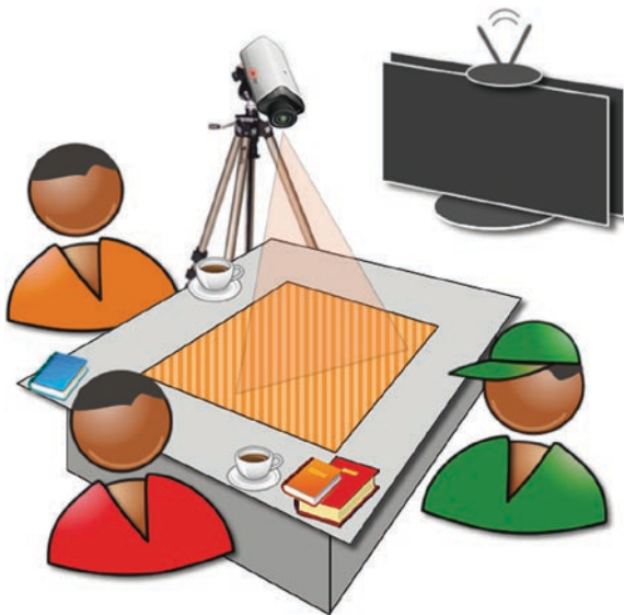
Fig. 9 Vision for interactive coffee tables: all the viewers may interact with the TV set using the same wide-area interface via simple hand movements on top of the video-sensitive area of the table. The interactive area is depicted in the center of the table with a darker color
