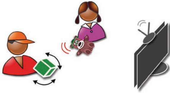
Fig. 8 Tangible devices such as special designed cubes or everyday objects such as toys may be used in order to map movements and rotations to shortcut commands for interfacing the TV-set
