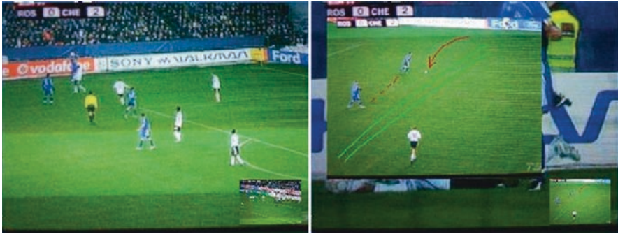
Fig. 2 A miniature image of the annotated frame is presented (left) to indicate that an ink note is available and is presented (right) if the user selects the square button on remote control; the triangle button resumes the playback
