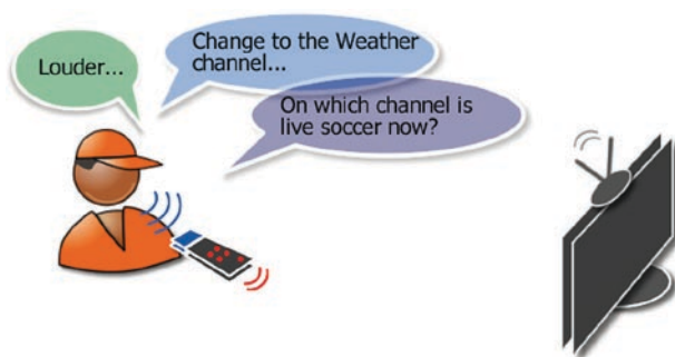
Fig. 4 Speech input is achieved by embedding microphones into the remote control. Special care is needed with regards to recognition accuracy, speaker variation, and environmental noise filtering. Speech comes as complementary rather than alternative interaction
