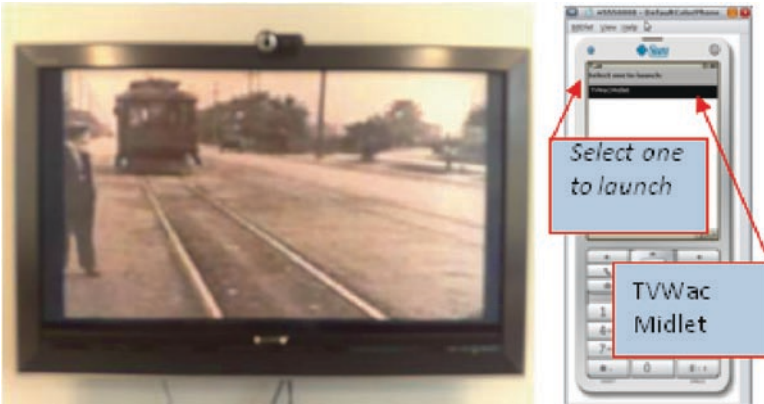
Fig. 5 While watching TV (left), users activate the WaC application in their mobile devices: the TVWacMidlet application, previously installed, is listed on the mobile device and can be initialized/executed (Select one to launch menu at the right upper corner), starting the search for available UPnP services
