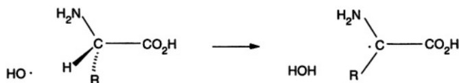
Figure 8.6. Abstraction of a hydrogen atom from the \alpha -C of an amino acid by hydroxyl radical has been investigated computationally.
