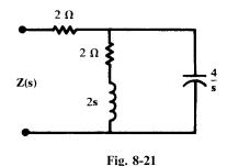
**8.11** Obtain the impedance  $\mathbf{Z}_{in}(\mathbf{s})$  for the circuit shown in Fig. 8-21 at (a)  $\mathbf{s} = 0$ , (b)  $\mathbf{s} = j4 \, \text{rad/s}$ , (c)  $|\mathbf{s}| = \infty$ .
