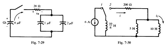
**7.16** In the circuit shown in Fig. 7-30, the switch is moved to position 2 at t = 0. Obtain the current  $i_2$  at t = 34.7 ms.
