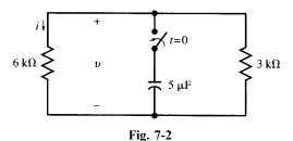
The equivalent resistance of the two parallel resistors is  $R = 2 \text{ k}\Omega$ . The time constant of the circuit is  $RC = 10^{-2} \text{ s}$ . The voltage and current in the 6-k $\Omega$  resistor are, respectively,
