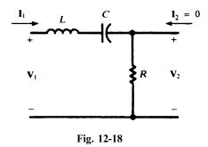
The circuit is said to be in *series resonance* (or *low-impedance resonance*) when  $\mathbf{Z}_{in}(\omega)$  is real (and so  $|\mathbf{Z}_{in}(\omega)|$  is a minimum); that is, when
