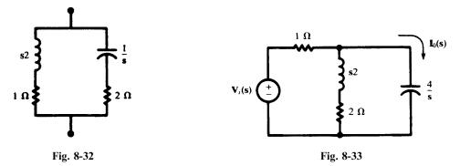
**8.32** The voltage source in the s-domain circuit shown in Fig. 8-33 has the time-domain expression
