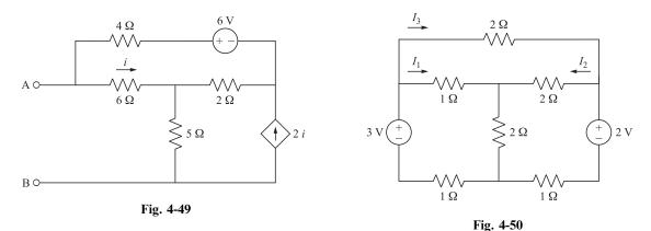
**4.43 Loop Current Method.** In the circuit of Fig. 4-50 write three loop equations using  $I_1$ ,  $I_2$ , and  $I_3$ . Then find the currents.
