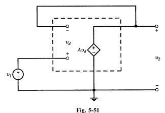
From Fig. 5-51 we have  $v_2 = Av_d$ . Applying KVL around the amplifier, obtain
