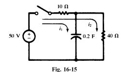
**16.17** In the two-mesh network shown in Fig. 16-15 there is no initial charge on the capacitor. Find the loop currents  $i_1$  and  $i_2$  which result when the switch is closed at t = 0.
