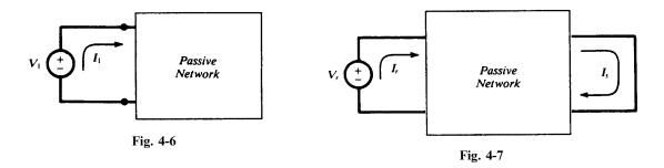
Thévenin too). The output resistance is found by dividing the open-circuited voltage to the short-circuited current at the desired node. The short-circuited current is found in Section 4.6.
