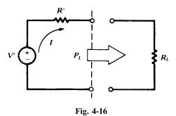
It is noted that the condition for maximum power transfer to the load is not the same as the condition for maximum power delivered by the source. The latter happens when  $R_L = 0$ , in which case power delivered to the load is zero (i.e., at a minimum).
