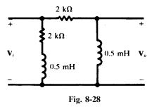
At  $\omega = 4 \times 10^6 \text{ rad/s}$ ,  $X_L = (4 \times 10^6)(0.5 \times 10^{-3}) = 2000 \,\Omega$ . Then,
