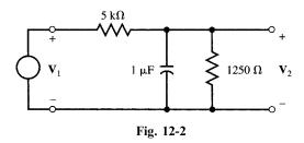
Alternative solution: First we find the Thévenin equivalent of the resistive part of the circuit,  $V_{\text{Th}} = V_1/5$  and  $R_{\text{Th}} = 1 \text{ k}\Omega$ , and then divide  $V_{\text{Th}}$  between  $R_{\text{Th}}$  and the 1- $\mu$ F capacitor to obtain (2a).
