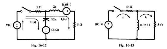
16.14 In the two-mesh network of Fig. 16-13, find the currents which result when the switch is closed.
