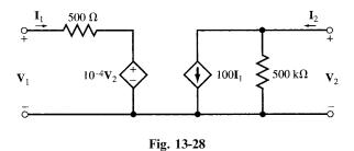
**13.20** The device H of Problem 13-19 is placed in the circuit of Fig. 13-29(a). Replace H by its model of Fig. 13-28 and find  $\mathbf{V}_2/\mathbf{V}_s$ .
