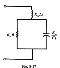
There are practical applications suggested by this brief exposure to magnitude scaling. For example, if the input current to a network were greater than it should be, a factor  $K_m = 10$  would reduce the current to 1/10 of the former value.
