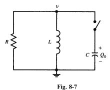
The transient response is easiest to visualize by assuming an initial charge  $Q_0$  on the capacitor and a switch that closes at t = 0. However, a step function voltage applied to the circuit will initiate the same transient response.
