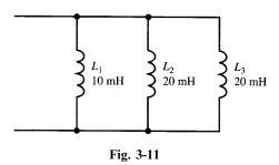
The two 20-mH inductances have an equivalent inductance of 10 mH. Since this is in parallel with the 10-mH inductance, the overall equivalent inductance is 5 mH. Alternatively,
