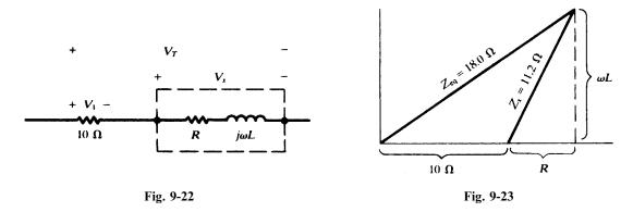
known. Given that f = 60 Hz,  $V_1 = 20 \text{ V}$ ,  $V_x = 22.4 \text{ V}$ , and  $V_T = 36.0 \text{ V}$ , find R and L.
