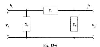
We apply KCL to the input and output nodes (for convenience, we designate the admittances of the three branches of the circuit by  $\mathbf{Y}_a$ ,  $\mathbf{Y}_b$ , and  $\mathbf{Y}_c$  as shown in Fig. 13-6). Thus,
