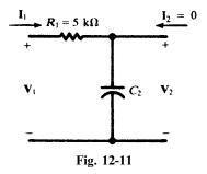
$$\mathbf{H}_{v\infty}(\omega) = \frac{1/j\omega C_2}{R_1 + (1/j\omega C_2)} = \frac{1}{1 + j(\omega/\omega_x)} \quad \text{where} \quad \omega_x \equiv \frac{1}{R_1 C_2} = \frac{2 \times 10^{-4}}{C_2} \quad \text{(rad/s)}$$
