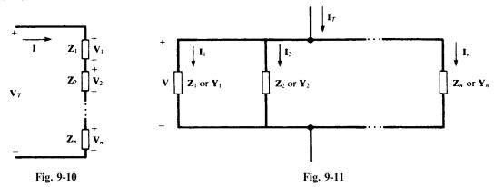
(2) Impedances in parallel (admittances in series) divide the total current in the inverse ratio of the impedances (direct ratio of the admittances):
