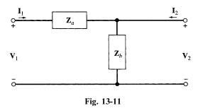
This is the simple lumped model of an incremental segment of a transmission line. From (29) we have
