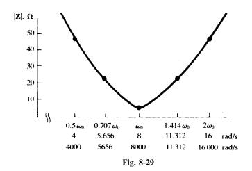
Thus, frequency scaling by a factor of 1000 results in the 5- $\Omega$  impedance value being attained at 8000 rad/s instead of 8 rad/s. Any other value of the impedance is likewise attained, after scaling, at a frequency 1000 times that at which it was attained before scaling. Consequently, the two graphs of  $|\mathbf{Z}(\omega)|$  differ only in the horizontal scale—see Fig. 8-29. (The same would be true of the two graphs of  $\theta_{\mathbf{Z}(\omega)}$ .)
