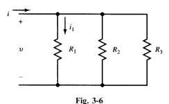
$$i = \frac{v}{R_1} + \frac{v}{R_2} + \frac{v}{R_3} \quad \text{and} \quad i_1 = \frac{v}{R_1}$$
