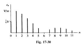
With the vertical axis positioned as shown, the wave is even and the series will contain only cosine terms and a constant term. In the period from  $-\pi$  to  $+\pi$  used for the evaluation integrals, the function is zero except from  $-\pi/6$  to  $+\pi/6$ .
