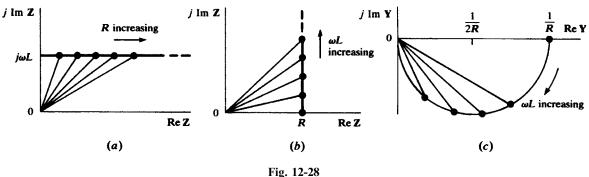
Note that for  $\omega L = 0$ ,  $\mathbf{Y} = (1/R)/0^{\circ}$ ; and for  $\omega L \to \infty$ ,  $\mathbf{Y} \to 0/-90^{\circ}$ . When  $\omega L = R$ ,
