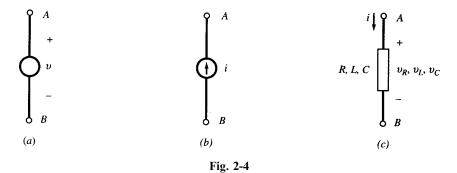
Similarly, a current source requires that a direction be indicated, as well as the function, as shown in Fig. 2-4(b). For passive circuit elements R, L, and C, shown in Fig. 2-4(c), the terminal where the current enters is generally treated as positive with respect to the terminal where the current leaves.
