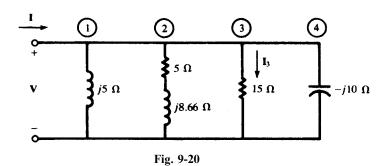
9.12 The total current I entering the circuit shown in Fig. 9-20 is 33.0 / -13.0° A. Obtain the branch current I<sub>3</sub> and the voltage V.
