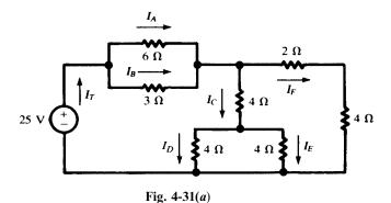
**4.15** Obtain the current in each resistor in Fig. 4-31(a), using network reduction methods.
