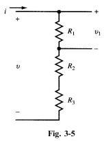
Since  $v_1 = iR_1$  and  $v = i(R_1 + R_2 + R_3)$ ,
