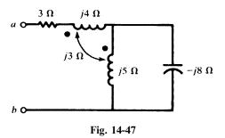
**14.38** Find the input impedance at terminals *ab* of the coupled circuit shown in Fig. 14-48. *Ans.* 1+j1.5  $\Omega$
