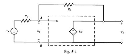
**EXAMPLE 5.3** Find  $v_2/v_s$  in Fig. 5-4 and express it as a function of the ratio  $b = R_1/(R_1 + R_2)$ . From the amplifier we know that
