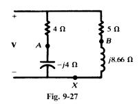
**9.17** In the parallel circuit shown in Fig. 9-27,  $V_{AB} = 48.3 / 30^{\circ} \text{ V}$ . Find the applied voltage V.
