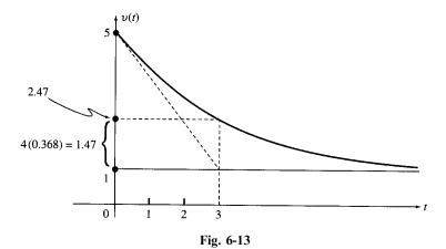
**EXAMPLE 6.23** The voltage  $v = V_0 e^{-|t|/\tau}$ ,  $\tau > 0$ , is connected to a capacitor. Find the current i in the capacitor. Sketch v and i for  $V_0 = 10 \, \text{V}$ ,  $C = 1 \, \mu \text{F}$ , and  $\tau = 1 \, \text{ms}$ .
