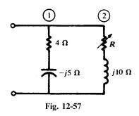
**12.32** Find *R* for resonance of the network shown in Fig. 12-57. Sketch the admittance locus diagram. *Ans.* Resonance cannot be achieved by varying *R*. See Fig. 12-58.
