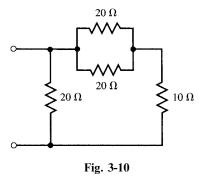
The two  $20-\Omega$  resistors in parallel have an equivalent resistance  $R_{\rm eq} = [(20)(20)/(20+20)] = 10\,\Omega$ . This is in series with the  $10-\Omega$  resistor so that their sum is  $20\,\Omega$ . This in turn is in parallel with the other  $20-\Omega$  resistor so that the overall equivalent resistance is  $10\,\Omega$ .
