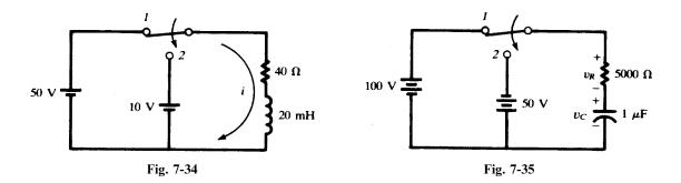
**7.22** The switch in the circuit shown in Fig. 7-35 is moved from 1 to 2 at t = 0. Find  $v_C$  and  $v_R$ , for t > 0.
