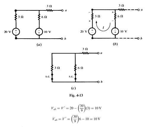
The resistance R' can be obtained by shorting out the voltage sources [Fig. 4.13(c)] and finding the equivalent resistance of this network at terminals ab:
