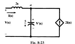
**8.14** Obtain **H(s)** for the network shown in Fig. 8-23, where the excitation is the driving current **I(s)** and the response is the voltage at the input terminals.
