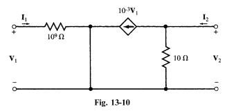
This is the simple model of a field effect transistor in its linear region of operation. To find the **g**-parameters, we first derive the terminal equations by applying Kirchhoff's laws at the terminals:
