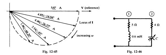
The semicircular admittance locus of branch 2 has the radius r = 1/2R = 0.125 S. The total admittance is the sum of the fixed admittance  $\mathbf{Y}_1$  and the variable admittance  $\mathbf{Y}_2$ . In Fig. 12-47, the semicircular locus is added to the fixed complex number  $\mathbf{Y}_1$ . The circuit resonance occurs at points a and b, where  $\mathbf{Y}_T$  is real.
