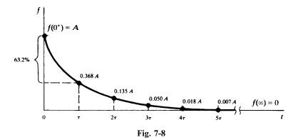
that is, at  $t = \tau$  the function is 36.8 percent of the initial value. It may also be said that the function has undergone 63.2 percent of the change from  $f(0^+)$  to  $f(\infty)$ . At  $t = 5\tau$ , the function has the value 0.0067A, which is less than 1 percent of the initial value. From a practical standpoint, the transient is often regarded as over after  $t = 5\tau$ .
