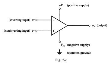
The output voltage  $v_o$  depends on  $v_d = v^+ - v^-$ . Neglecting the capacitive effects, the transfer function is that shown in Fig. 5-7. In the linear range,  $v_o = Av_d$ . The open-loop gain A is generally very high.  $v_o$  saturates at the extremes of  $+V_{cc}$  and  $-V_{cc}$  when input  $v_d$  exceeds the linear range  $|v_d| > V_{cc}/A$ .
