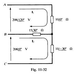
The method of Example 11.7 could be applied here and one node-voltage equation solved. However, the mesh currents  $I_1$  and  $I_2$  suggested in Fig. 11-32 provide another approach.
