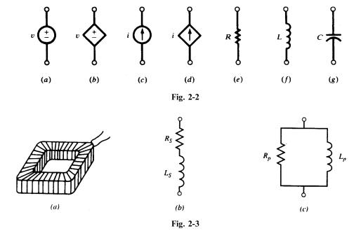
In general, a coil can be represented by either a series or a parallel arrangement of circuit elements. The frequency of the applied voltage may require that one or the other be used to represent the device.
