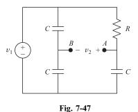
**7.46** In the circuit of Fig. 7-47, find the differential equation relating  $v_2$  to  $v_1$ . Compare with the circuit of Fig. 7-45(a) of Example 7.17.
