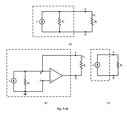
(a) In the direct connection, Fig. 5-44(a),  $i_l = i_s R_s / (R_s + R_l)$ , which varies with  $R_l$ . (b) In Fig. 5-44(b), the op amp forces  $v_B$  to zero causing the current in  $R_s$  to become zero. Therefore,  $i_l = i_s$  which is now independent of  $R_l$ . The op amp circuit converts the practical current source to an ideal current source. See Figure 5-44(c).
