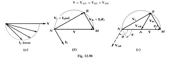
Because  $I_2$  lags  $V_{BN}$  by 90°,  $V_{BN}$  and  $V_{MB}$  are perpendicular for all values of L in Fig. 12-50(b). As L varies from 0 to  $\infty$ , point B moves from N toward M along the semicircle. Figures 12-49 and 12-50(b) are superimposed in Fig. 12-50(c). It is clear that  $V_{AB}$  is a radius of the semicircle and therefore,
