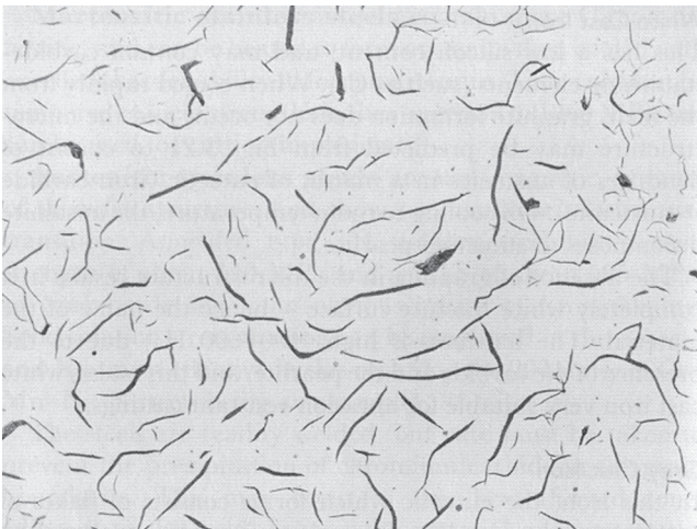
3.28 Optical micrograph of grey cast iron (unetched) \times 500 .
