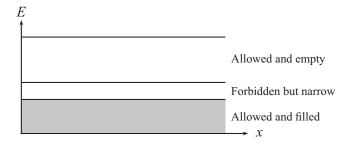
**Figure 3.4** Energy band structure for a semiconductor.
