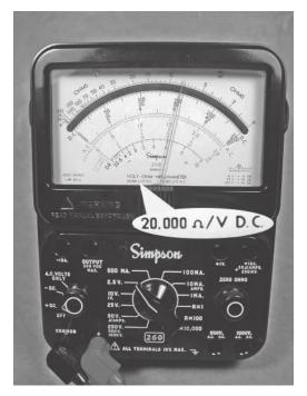
**Figure 1.23** Impedance specification for a typical analog meter.
