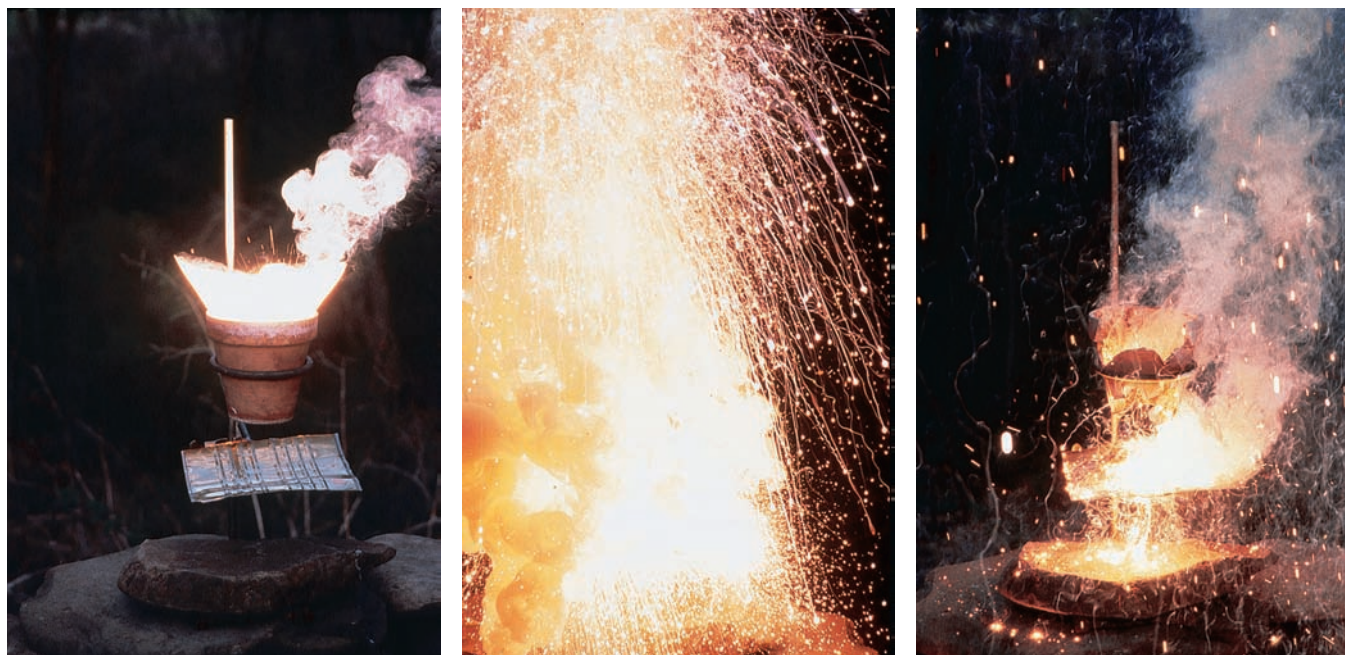
FIGURE 12.16 The thermite reaction, 2 \text{Al}(s) + \text{Fe}_2\text{O}_3(s) \longrightarrow 2 \text{Fe}(s) + \text{Al}_2\text{O}_3(s) , is among the most exothermic of all reactions, liberating 16 kJ of heat for every gram of aluminum that reacts. (a) A piece of burning magnesium acts as a source of ignition when inserted into a pot containing a finely divided mixture of aluminum powder and iron(III) oxide. (b) After the ignition, the reaction continues on its own. (c) Enough heat is generated to produce molten iron, which can be seen flowing out of the broken pot onto the protective mat and the bottom of the stand.
