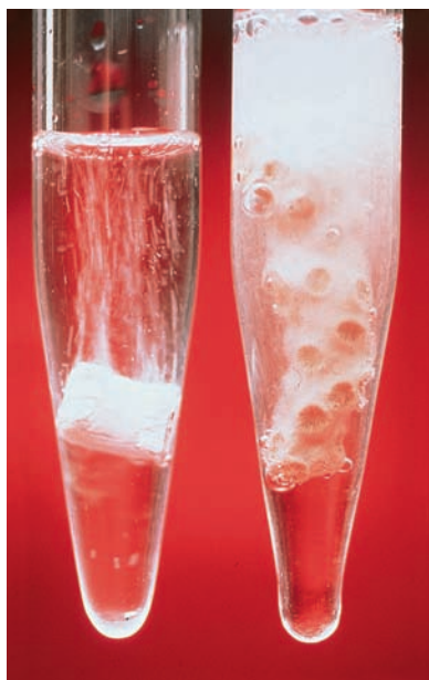
FIGURE 9.4 The calcium carbonate in a piece of chalk reacts with an aqueous solution of hydrochloric acid to produce bubbles of carbon dioxide.
