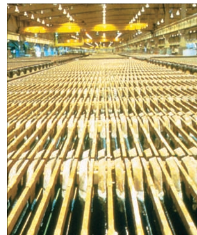
FIGURE 17.30 Electrolytic refining of copper. Many slabs of impure copper (anodes) alternating with thin sheets of pure copper (cathodes) are immersed into a dilute acidic solution of \text{CuSO}_4 . Copper metal oxidized from the impure anodes enters the solution as \text{Cu}^{2+} ions that migrate to the cathodes where they plate out as copper metal of higher purity.
