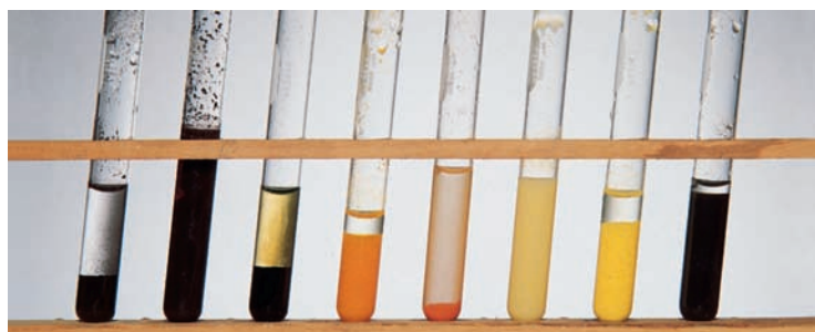
FIGURE 16.19 These sulfides are insoluble at pH 1, so they can be separated out of a mixture containing other, more soluble sulfides. From left to right, they are PbS, \text{Bi}_2\text{S}_3 , CuS, CdS, \text{Sb}_2\text{S}_3 , \text{SnS}_2 , \text{As}_2\text{S}_3 , and HgS. The precipitates occupy the lower part of the test tubes; in the 2nd and 6th from the left, the precipitate appears as a dispersion of fine particles. The colored bands observed at each meniscus are refracted images of the colored solids at the bottom of each tube.
