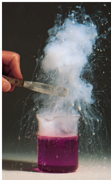
FIGURE 16.15 The acidity of metal ions is illustrated by the vigorous reaction of anhydrous \text{AlCl}_3 with water to generate hydrated aluminum oxides, \text{HCl}(aq) , and heat. The \text{HCl} turns the indicator, bromocresol red, to its red acid form.
