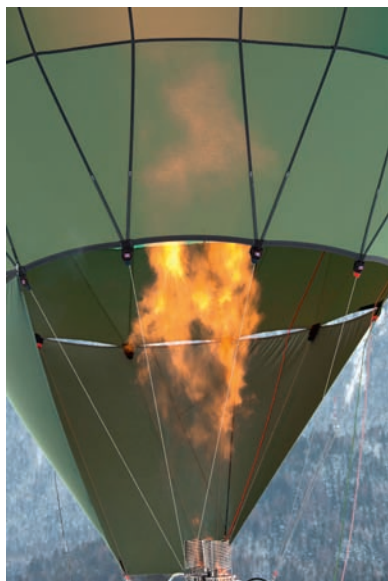
FIGURE 9.10 In a hot-air balloon, the volume remains nearly constant (the balloon is rigid) and the pressure is nearly constant as well (unless the balloon rises very high). Thus, n is inversely proportional to T ; as the air inside the balloon is heated, its amount decreases and its density falls. This reduced density gives the balloon its lift.
