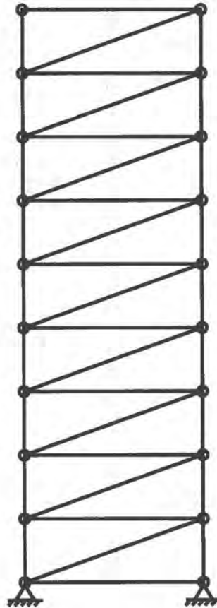
Figure 2-62 Plate Wall Diagonal Tension Brace Model
