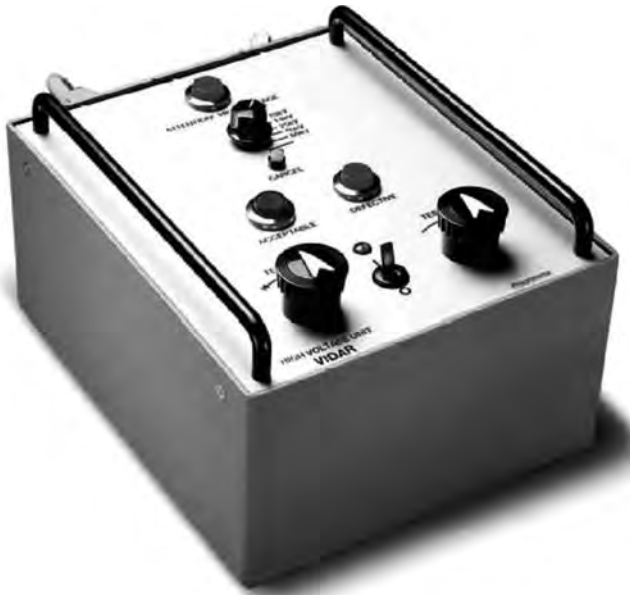
FIGURE 7.15 A DC Megger Vidar instrument. (Courtesy of Megger/Programma, Valley Forge, PA.)
