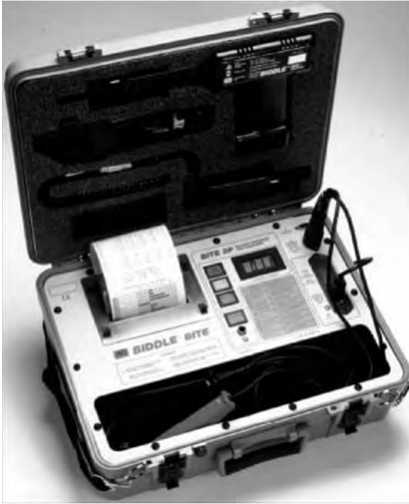
FIGURE 7.33 Battery impedance tester (BITE). (Courtesy of Megger, Inc., Dallas, TX.)
