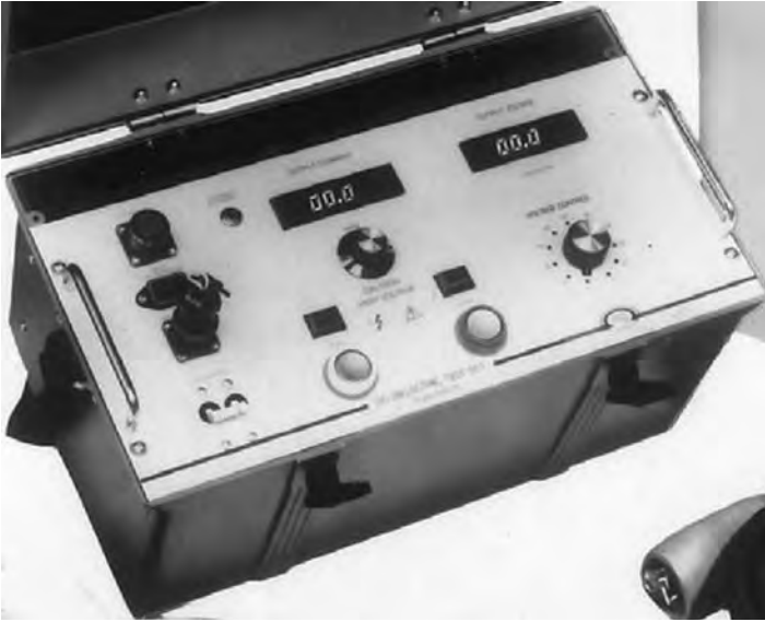
FIGURE 2.8 DC hi-pot test set, 70 kV. (Courtesy of Megger, Inc., Valley Forge, PA.)
