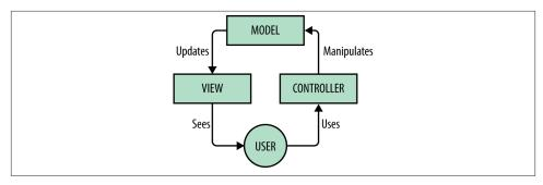
Figure 1-3. How MVC works
