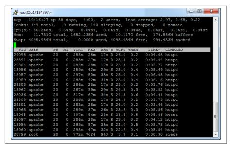
Figure 16-8. Using the top command to figure out how much memory is available
