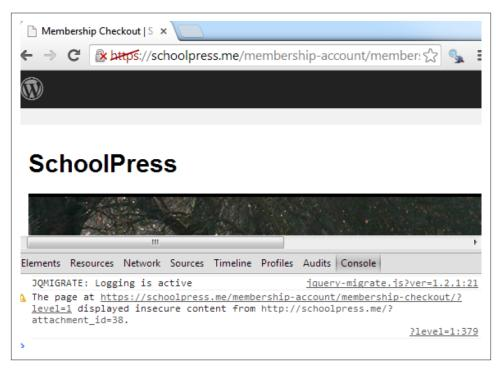
Figure 15-5. An SSL error in the Chrome Developer Tools Console. Use the Chrome Developer Tools Console to find SSL errors, or use the Nuclear Option to avoid them.
