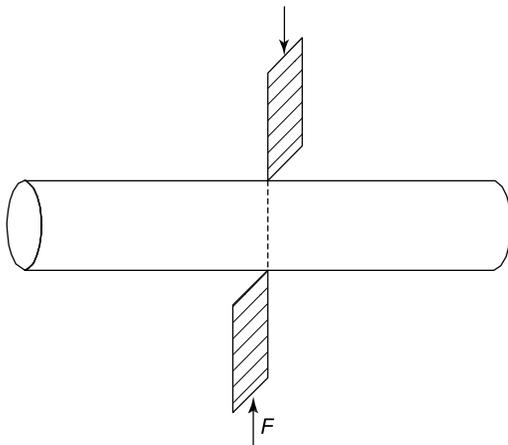
Figure 7.3 Shearing action
