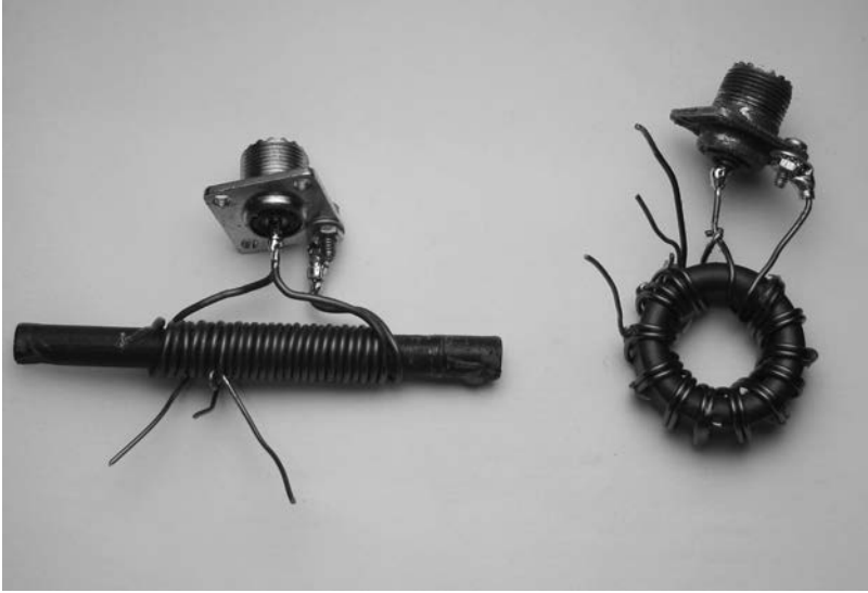
Figure 7-28 This photo shows examples of two tapped bifilar transformers with impedance ratios approximating 1:1.3. Each transformer has taps between 1:3.2 and 1:4.
