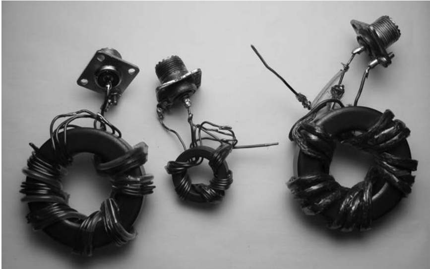
Figure 7-11 The transformer on the left matches 100 to 150 \Omega . The center transformer matches 50 to 32 \Omega and has response 150 MHz wide. The transformer on the right uses low impedance cable and has 5 kW capability.
