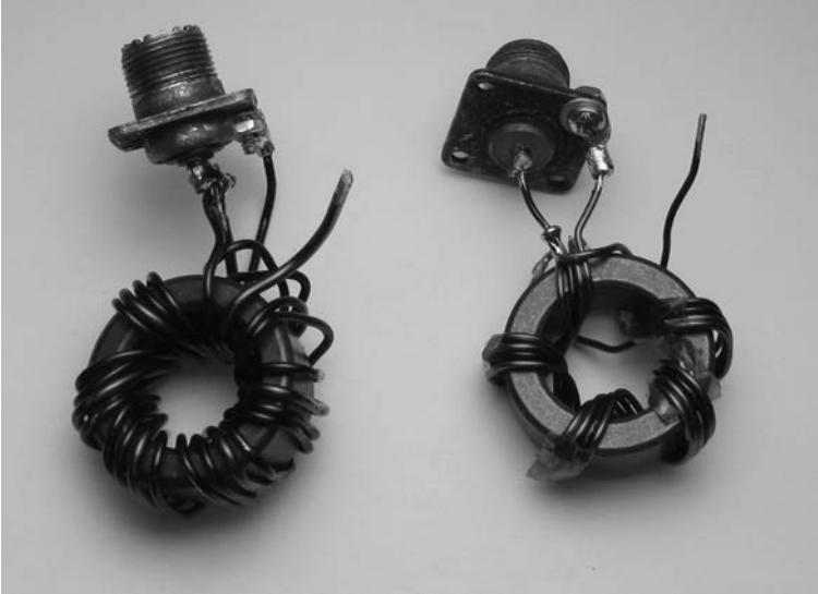
Figure 7-27 This photo shows examples of two quadrifilar 1:1.78 ratio transformers. They both implement the schematic of Figure 7-26(b) which favors matching 28\ \Omega to 50\ \Omega . The left transformer is rated at 2 kW because of the use of no. 12 wire. The one on the right is rated at 1 kW continuous power.
