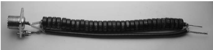
Figure 11-3 Photo shows construction of a 4:1 equal delay transformer using a linear configuration and “one turn” of coax cable through many ferrite beads.
