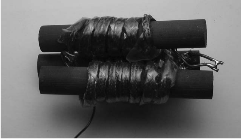
Figure 9-15 Photo shows a 1:9 low impedance transformer designed for the 50:5.56 \Omega range.
