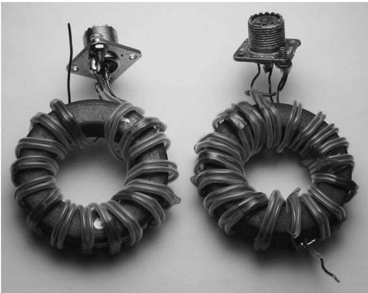
Figure 9-9 Two 1:4 baluns for the 50:200 \Omega level are shown: (Left) Ruthroff design. (Right) Guanella design with both transmission lines on the same core.
