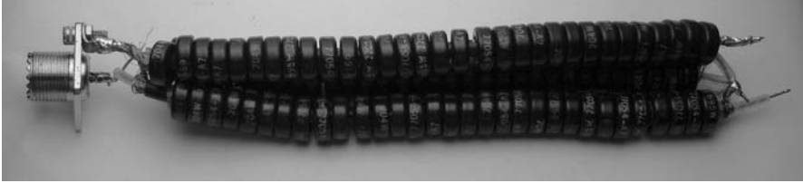
Figure 11-8 Photo shows the implementation of the circuit of Figure 11-7 to create a 1:2.25 balun.
