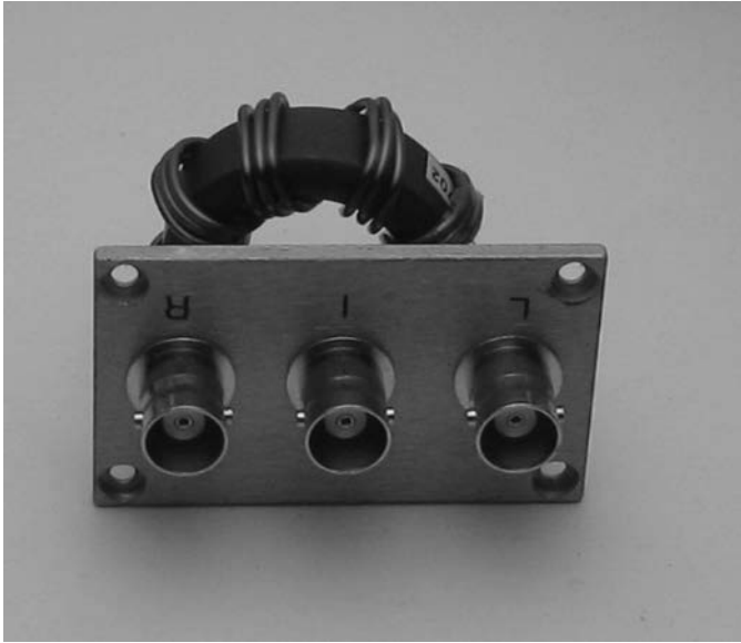
Figure 8-12 A tapped trifilar transformer that is designed to give ratios between 1:4 and 1:9.
