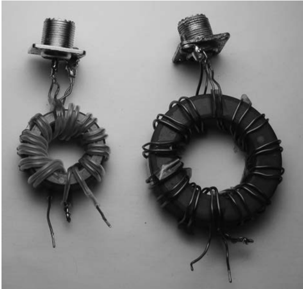
Figure 9-13 This photo shows two high impedance Guanella transformers that use one core for both transmission lines.
