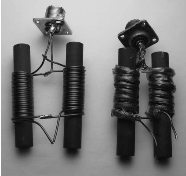
Figure 9-14 Photo shows two low impedance Guanella transformers: (Left) Parallel line. (Right) Low impedance coax.
