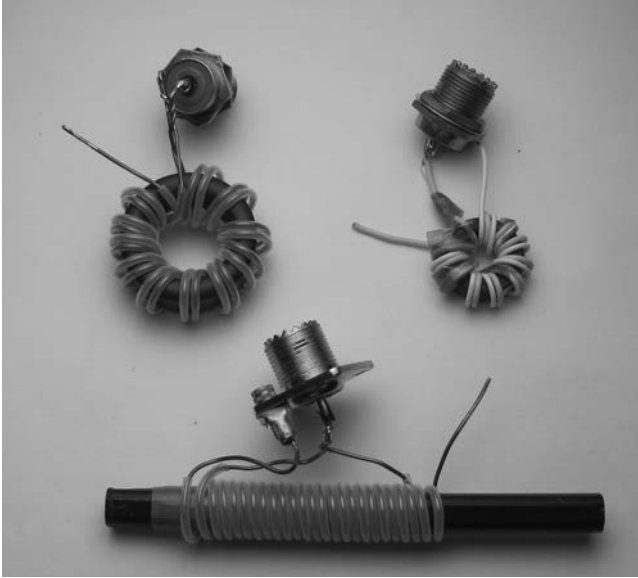
Figure 6-8 50:200 Ruthroff transformers require additional insulation.
