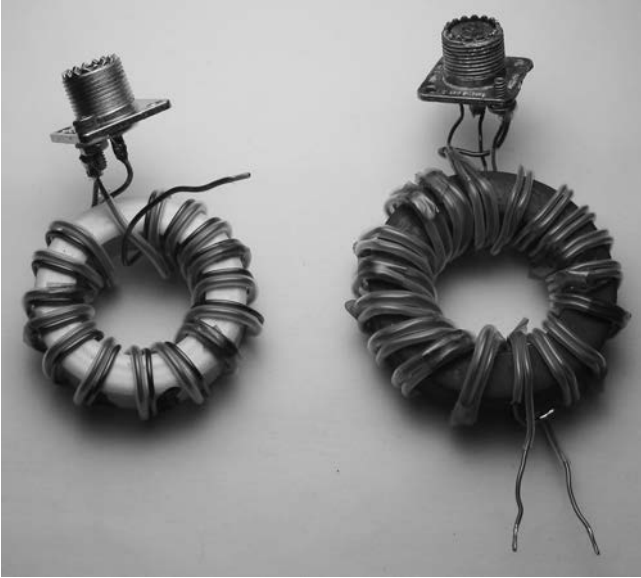
Figure 9-11 Photo used to study the relative merits of (left) a transformer using powdered iron toroid, as found in some antenna tuners, and (right) Guanella transformer using a single ferrite core.
