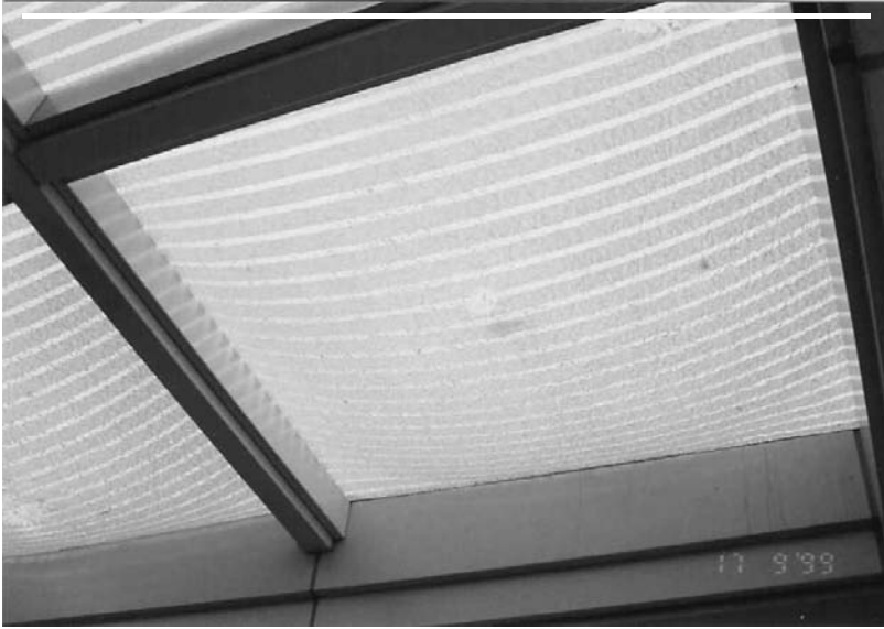
FIGURE 29.9 Laminated glass when it is broken.
