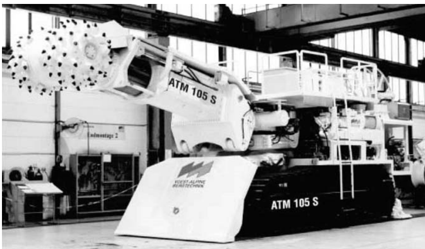
FIGURE 28.7 Roadheader with double rotating cutterhead and gathering apron (© Sandvik 2000, with permission).
