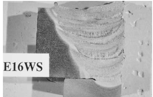
FIGURE 34.20 Fracture surface and weld cross-section from moment-frame connection that fractured in the Northridge Earthquake showing a typical crack that originated at the backing bar notch.
