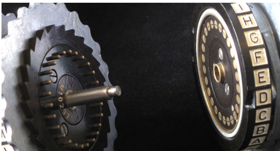
Figure 1-2. A pair of Enigma rotors used for calibrating the Enigma machine's transmission configuration, an analog equivalent of changing a digital cipher's primary key
