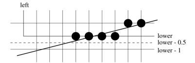
Figure 3.16 Finding the pixel where a line enters the clipping rectangle
