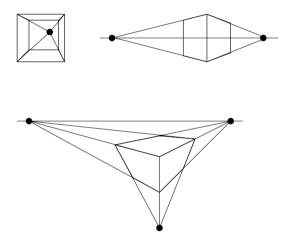
Figure 5.12 One-, two- and three-point perspective projections
