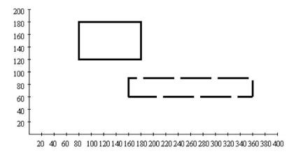
Figure 2.13 Scaling applied to a rectangle
