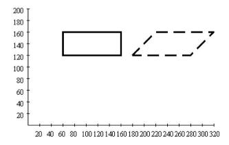
Figure 2.15 A shear transformation applied to a rectangle
