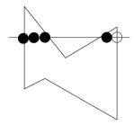
Figure 4.2 Scan line technique for filling polygons
