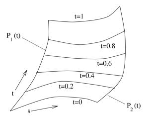
Figure 6.17 A parametric freeform surface
