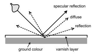
Figure 8.7 Diffuse and specular reflection
