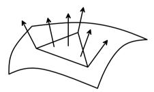
Figure 8.13 Interpolated normal vectors for Phong shading
