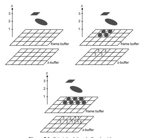
**Figure 7.5** Principle of the z-buffer algorithm
