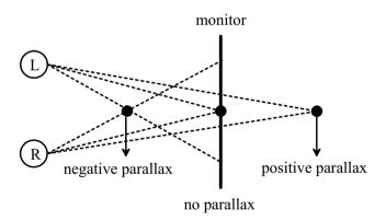
Figure 9.5 Parallax for stereoscopic viewing
