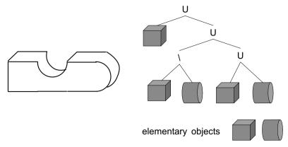
**Figure 6.9** An object that was constructed using elementary geometric objects and set-theoretic operations shown on the right
