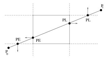
Figure 3.15 Potential intersection points with the clipping rectangle
