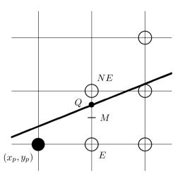
**Figure 3.3** The two candidates for the next pixel for the line drawing algorithm
