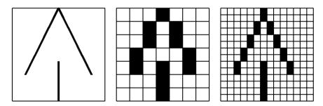
Figure 2.2 The tip of an arrow drawn as raster graphics in two different resolutions
