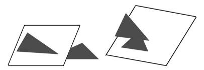
**Figure 7.11** Does one polygon lie completely in front or behind the plane induced by the other?
