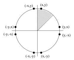
Figure 3.17 Exploiting symmetry for drawing circles
