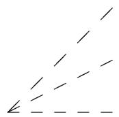
Figure 3.9 Different dash lengths for the same bitmask
