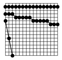
Figure 3.2 Lines resulting from the naïve line drawing algorithm
