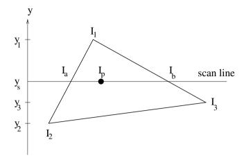
Figure 8.12 Scan line technique for the computation of Gouraud shading
