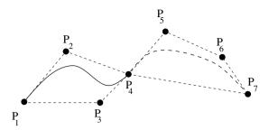
**Figure 6.15** B-spline with knots  $P_1, P_4, P_7$  and inner Bézier points  $P_2, P_3, P_5, P_6$
