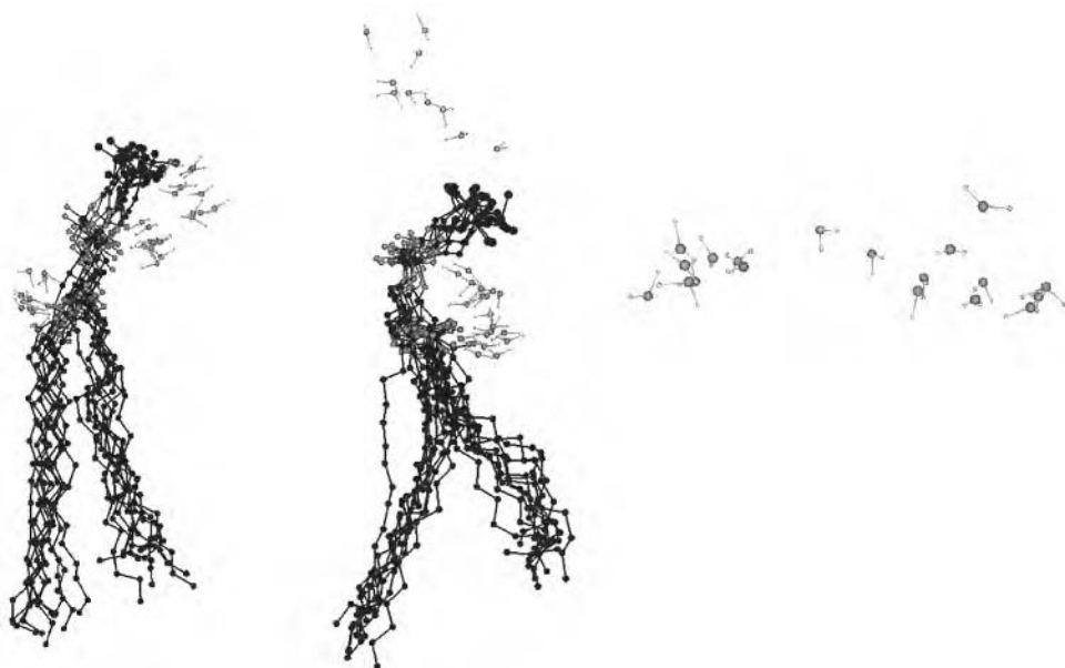
Figure 8 Configurations of lipid and water molecules spanning a 100 ps interval during an MD simulation of a DPPC bilayer. The two left-hand panels show 10 configurations of two different lipids and three of their associated water molecules (one N-bound, one P-bound, and one CO-bound). The right-hand panel shows 20 configurations of a “bulk” water molecule in the interlamellar space of a bilayer stack. (From Ref. 55.)
