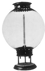
Jablotschkow's version of the arc lamp, exposed and with glass bulb.
