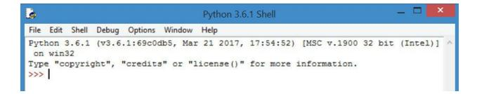
The Python Shell allows us to use Python in interactive mode. This means we can enter one command at a time. The Shell waits for a command from the user, executes it and returns the result of the execution. After this, the Shell waits for the next command.
