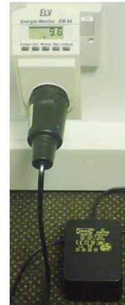
Figure 22.1. An awful AC lamp-adaptor from IKEA – the adaptor uses nearly 10 W even when the lamp is switched off!
