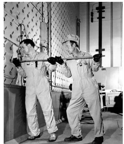
Figure 24.3. Workers push uranium slugs into the X-10 Graphite Reactor.
