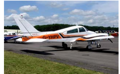
Figure C.9. Cessna 310N: 60 kWh per 100 passenger-km. A Cessna 310 Turbo carries 6 passengers (including 1 pilot) at a speed of 370 km/h. Photograph by Adrian Pingstone.
