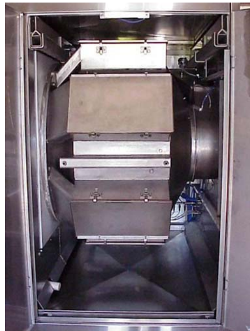
FIGURE 34.22 Exhaust plenum on the exterior of a partially perforated coating drum.
