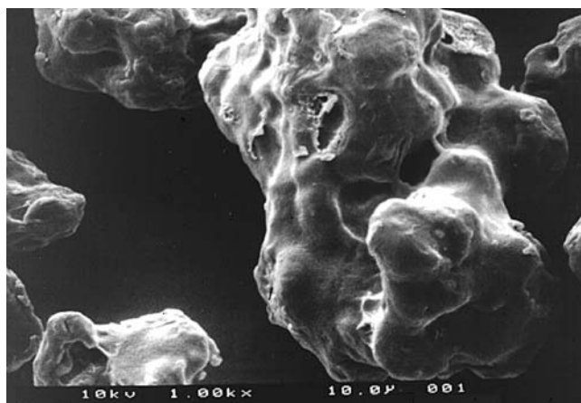
FIGURE 35.10 Very fine particles coated with a moisture barrier using the HS Wurster process (1000× magnification).
