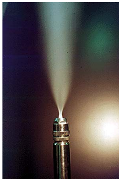
FIGURE 35.3 Spray nozzle and spray pattern (using water).
