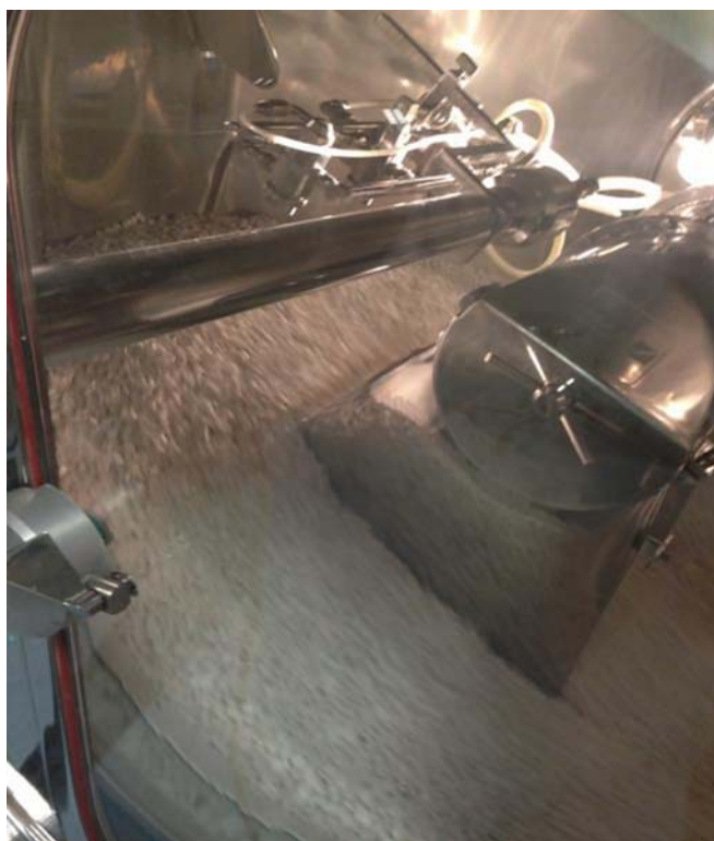
FIGURE 34.1 A solid coating pan fitted with immersion sword air-flow enhancement.
