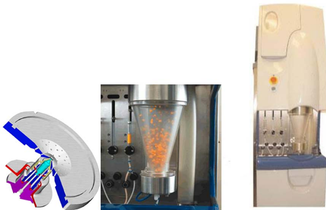
FIGURE 29.3 Cutaway view of the liquid nozzle and gas distribution plate, tablet movement inside the coating chamber, and the SUPERCELL coater general appearance. Source: Courtesy GEA Niro Pharma Systems.
