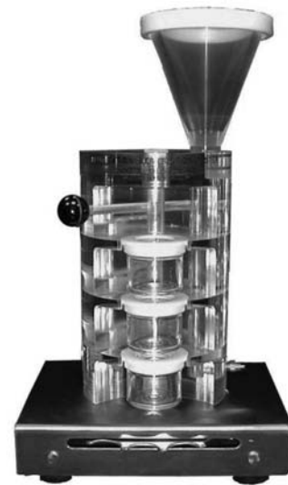
FIGURE 26.24 Fluidization segregation tester (controls not shown). Source: Photo provided courtesy of Jenike & Johanson, Inc.
