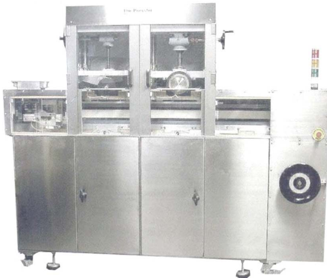
FIGURE 33.41 Presster—rotary tablet press replicator. Source: Photo courtesy of MCC—Metropolitan Computing Corporation, East Hanover, NJ.
