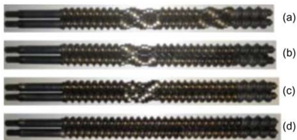
FIGURE 31.22 Different screw designs used to evaluate indomethacin-eudragit E ASD. 61
