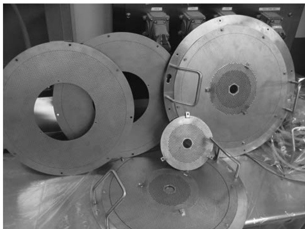
FIGURE 35.5 Up- and down-bed orifice plates for an 18" HS Wurster coater. Source: Photograph courtesy from Glatt Air Techniques, Inc.
