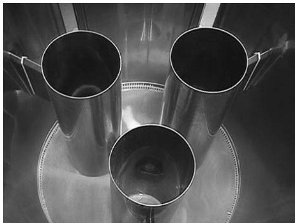
FIGURE 35.25 Inside view of 32" HS Wurster coater. Source: Photograph courtesy from Glatt Air Techniques, Inc.
