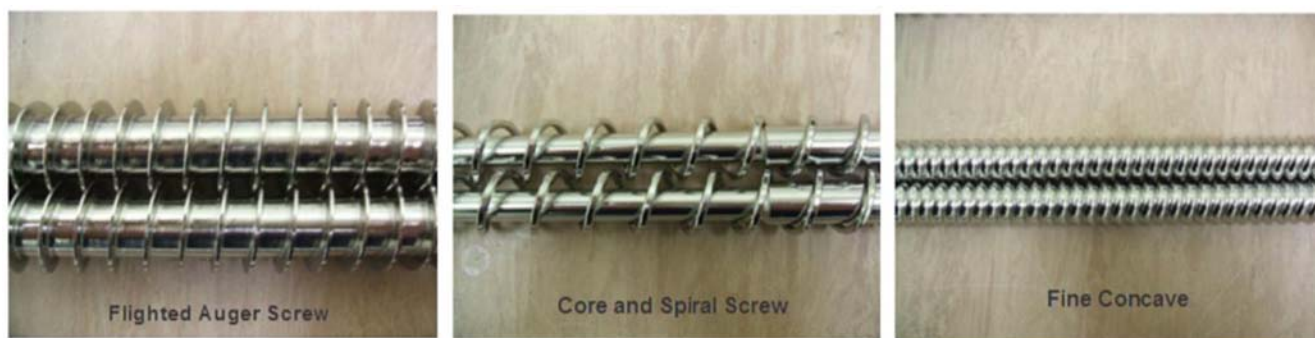
FIGURE 31.33 Transport screws used in K-Tron LIW feeder. 130
