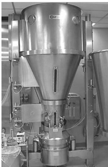
FIGURE 35.1 Glatt model GPCG-60 fluid-bed processor fitted with an 18" HS Wurster insert. Source: Photograph courtesy from Glatt Air Techniques, Inc.
