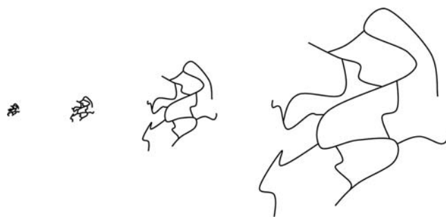
FIGURE 7.3 Depending upon the length and the flexibility of chain segments between covalent cross-links, a cross-linked polymer may be a very rigid and nonswelling solid (short, rigid segments between cross-links) or very highly swelling (low cross-link density between very flexible and solvent compatible segments) under the appropriate solvent conditions. In some cases, for example with a change of pH from highly acid to neutral or basic for a cross-linked polyacrylic acid system, conversion between collapsed and highly swollen states is readily and reversibly accomplished.
