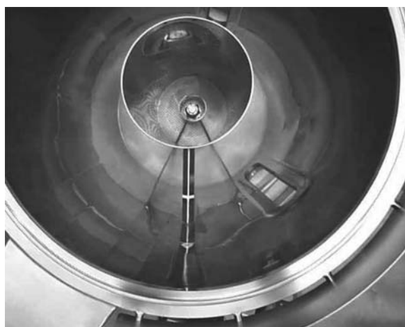
FIGURE 35.2 18" HS Wurster coater—inside view showing spray nozzle, HS nozzle surround, and partition. Source: Photograph courtesy from Glatt Air Techniques, Inc.
