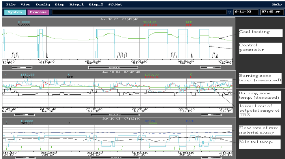
Fig. 4. The setpoint of burning zone temperature is properly adjusted after learning
