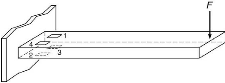
FIGURE 2.11 Cantilever beam with four strain gages.
