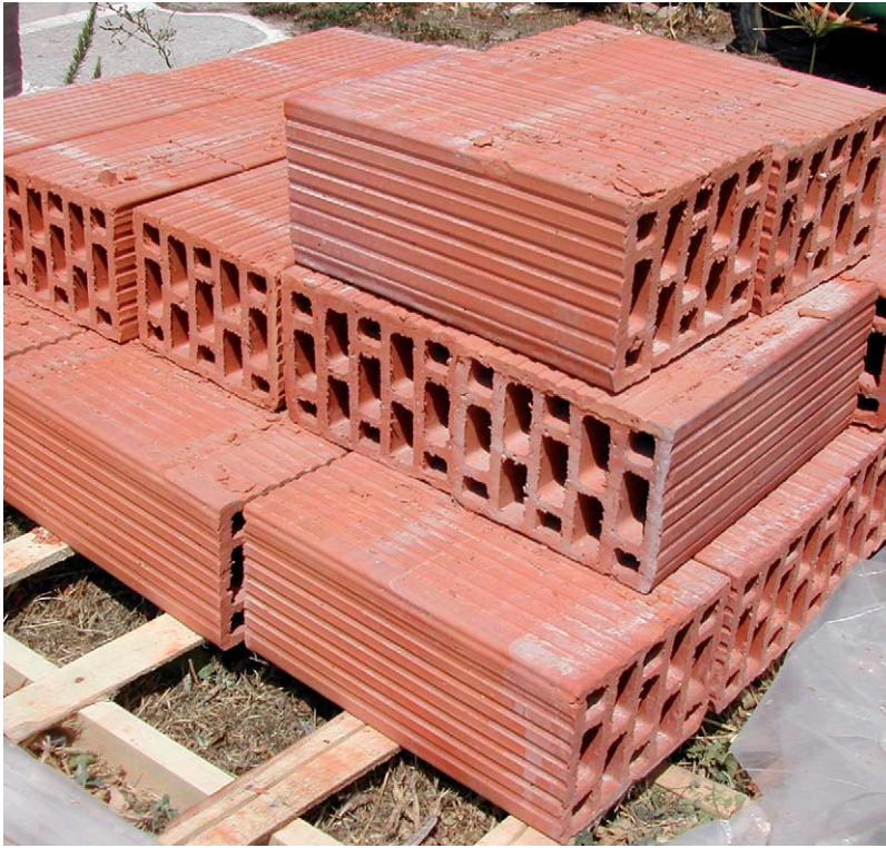
Fig. 2.8 Continued. Hollow clay blocks in Greece. Photograph: Arthur Lyons
