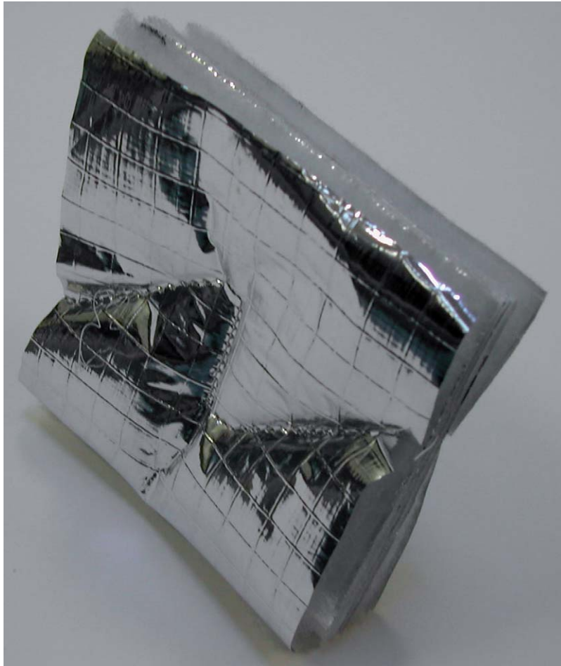
Fig. 13.3 Multi-layer aluminium foil insulation system
