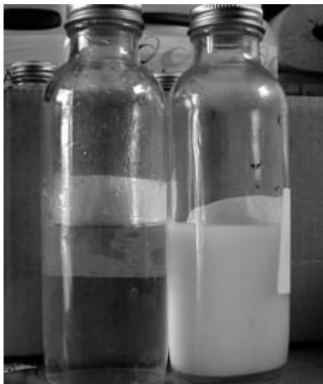
Fig. 3.5 The effect of adding coagulant and polymer during the treatment of wastewater.
