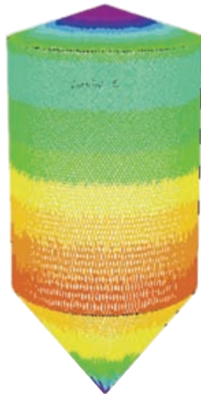
Plate 3 SaniJet 25 – full pattern of cleaning liquid distribution build-up. Reproduced by permission of Alfa Laval Tank Equipment A/S, Ishoej, Denmark.
