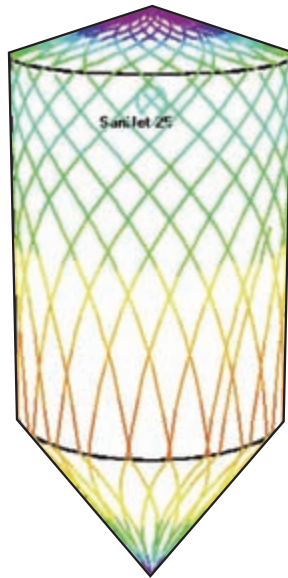
Plate 2 SaniJet 25 – pattern of cleaning liquid distribution build-up – first cycle. Reproduced by permission of Alfa Laval Tank Equipment A/S, Ishoej, Denmark.
