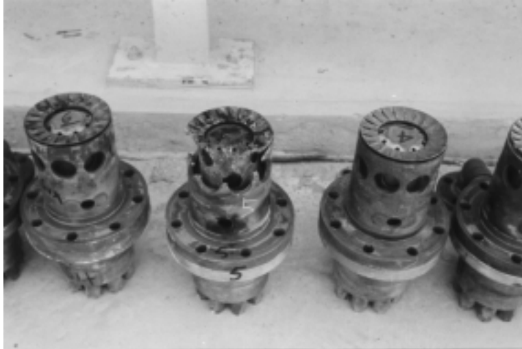
Figure 12-13. Burnt fuel nozzles from can-annular combustor. 55,000 horsepower gas turbine-generator with less than 10,000 operating hours.
