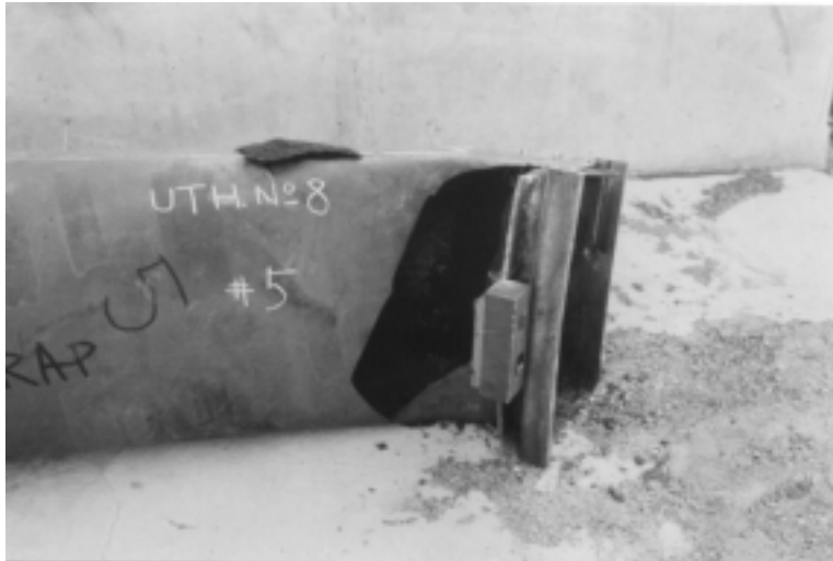
Figure 12-11. Can-annular combustor transition piece failure due to brittle fatigue due to fretting. 55,000 horsepower gas turbine-generator with less than 10,000 hours operation.
