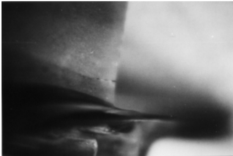
Figure 12-21. Trailing edge crack in the first stage turbine nozzle trailing edge. 5,000 horsepower gas turbine-compressor drive unit with less than 7,000 hours operation.
