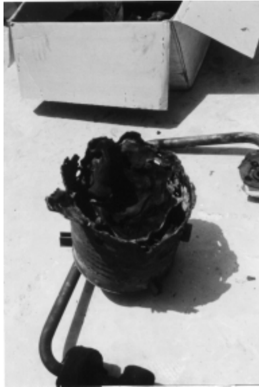
Figure 12-9. Can-annular combustor failure due to liquid carry-over in the fuel gas. 30,000 horsepower gas turbine-pump drive unit with less than 24,000 operating hours.
