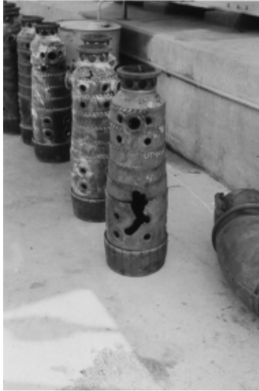
Figure 12-10. Can-annular combustor failure (burning and cracking) due to liquid mist in the fuel gas. 55,000 horsepower gas turbine-generator unit with less than 10,000 operating hours.
