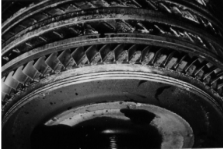
Figure 12-7. View of last stage compressor blades with contamination evident on and between blades. 5,000 horsepower gas turbine-generator unit after 44,500 hours operation.
