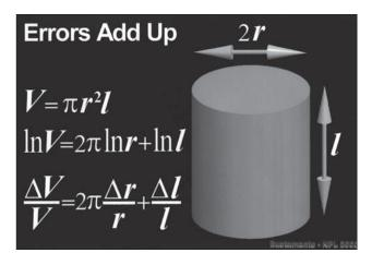
Figure 2. Error estimation for quantities that are derived from formulas. The example is given for the calculation of the volume, V, of a cylinder (e.g., NPC) with the measured values for its radius and length, r and l, respectively. Errors never cancel each other. Instead, they add up.
