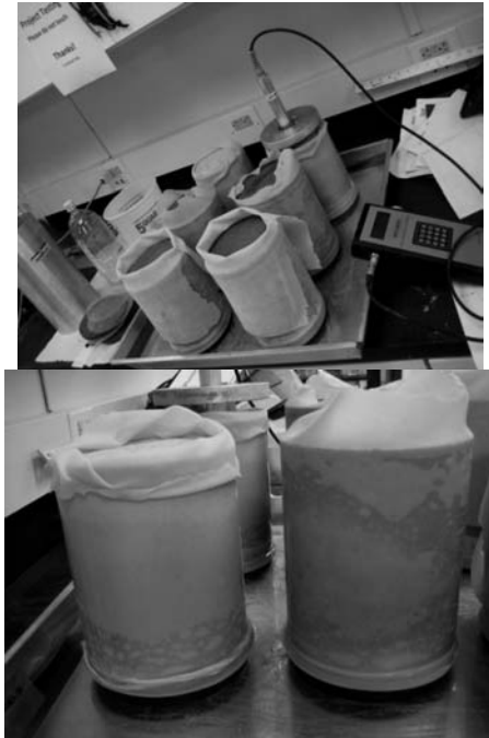
FIG.1. Illustration of the tube suction test using percometer
