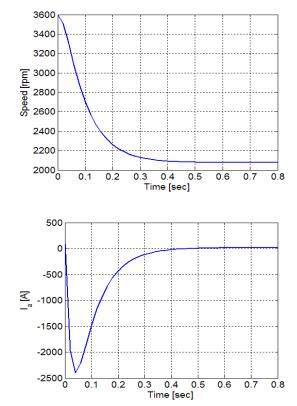
Note that this simulations indicates that such operation should not be attempted with this motor. The huge armature current which results would clearly overheat and probably damage the armature winding.
