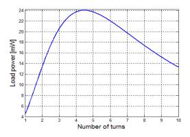
The maximum power will be supplied to the load resistor when its impedance, as reflected to the primary of the ideal transformer, equals that of the source (1.5 k $\Omega$ ). Thus the transformer turns ratio N to give maximum power must be
