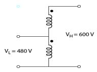
Part (b): The rated current of the high voltage terminal is equal to that of the 120-V winding,  $I_{\text{rated}} = 10^4/120 = 83.3 \text{ A}$ . Hence the kVA rating of the transformer is  $600 \times 83.3 = 50 \text{ kVA}$ .
