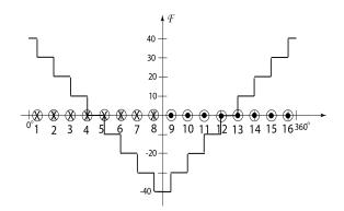
With one phase open-circuited, the motor becomes equivalent to a single-phase motor, with equal positive- and negative-traveling mmf waves.
