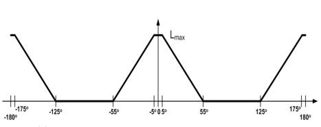
Part (b): The inductance changes from 0 to  $L_{\max}$  as the rotor rotates through angle  $\beta$  and thus
