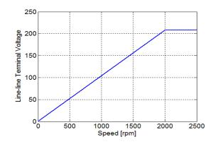
Part (d): At 1500 r/min,  $f_{\rm e} = 50$  Hz,  $X_{\rm s} = 1.76 \ \Omega$ ,  $E_{\rm am} = 138.8$  V, line-line and the terminal voltage must be limited to  $V_{\rm t} = 156$  V, line-line. For any given value of power angle  $\delta$ , the terminal current will be equal to
