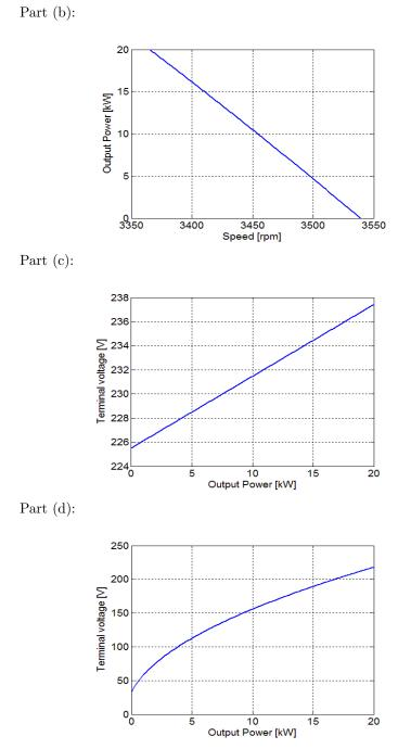
From a comparison of the results of Parts (c) and (d), one sees that this operation appears to be quite feasible but it requires a large variation in terminal voltage as compared to the case where the shunt field voltage is held constant.
