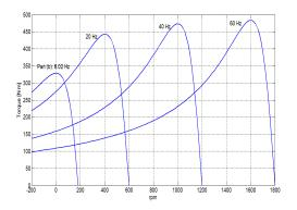
Part (b): f = 6.02 Hz which will produce a starting torque of 329 N·m.
