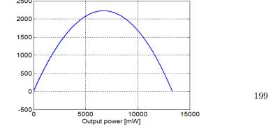
A MATLAB solution shows that the output power is equal to 2 W at 4624 r/min at which speed the efficiency is 32.8% and at 8845 r/min at which speed the efficiency is 56.0%.
