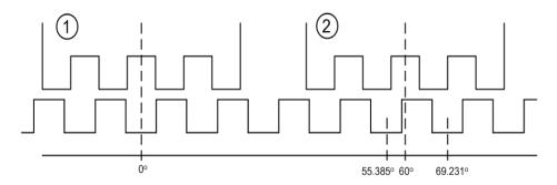
From the figure, we see that if phase 1 is turned off and phase 2 is energized, the rotor will rotate  $4.615^{\circ}$  degrees to the right (clockwise) to align with the phase-2 pole. Similarly, if phase 3 is excited after phase 1 is turned off, the rotor will rotate  $4.615^{\circ}$  degrees to the left (counterclockwise).
