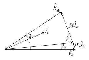
(ii) Working in per-unit,  $V_{\infty} = 1.0$ ,  $V_{\rm t} = 26.3/26 = 1.012$  and P = 375/550 = 0.682. The base impedance is  $Z_{\rm base} = 26^2/550 = 1.229 \ \Omega$  and thus  $X_{\infty} = 0.35$  per unit. From Eq. 5.43
